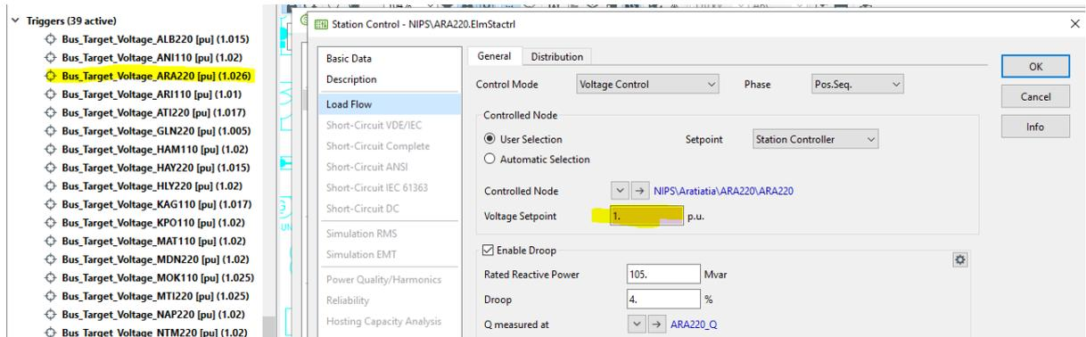
Note that the final voltage of the controlled bus may not be the value of the trigger because of the droop setting of the station controller – refer to the Station Controller Technical Reference for more details regarding droop (available through the PowerFactory help menu).
